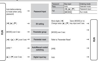
01) In case of TK4S model, short press of [MODE] key replaces [A/M] key function.
