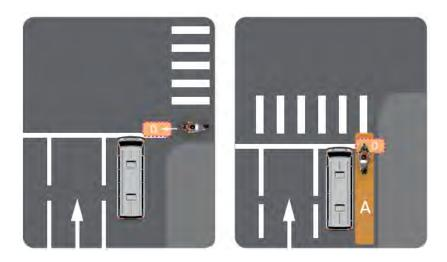
♦ When you turn on the turn signal light and wish to make a turn, this system will increase its alert level. If the red wide-turn assist indicator on the dashboard flashes and continues to emit short warning beeps, it indicates that there may be a vehicle in the following zones: Please slow down and check your surroundings before safely continuing.
