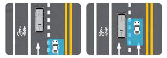
◆ If the blind spot indicator on the left A-pillar lights up or flashing, it indicates that there is a vehicle entering the left side of your vehicle or a vehicle approaching from the rear left side at high speed. Please slow down and check your surroundings before safely continuing.
