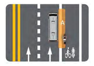
◆ If the red wide-turn assist indicator lights up when you start accelerating your vehicle after stopping at the traffic light, it indicates that there may be a vehicle on the right or front right side of your vehicle. Please be sure to stop driving to avoid accidents. If the red wide-turn assist indicator flashes and continues to emit short warning beeps
