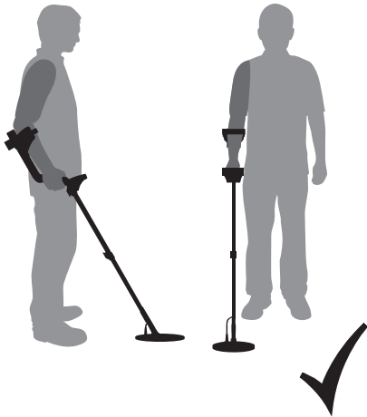
Shaft is the correct length
