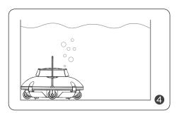
The device will automatically move to stop by the wall when finishing cleaning or battery low.
