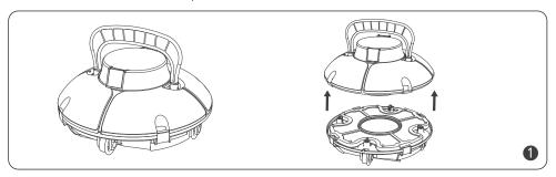
Unclip cover fasteners, and remove the top cover from the cleaner.
