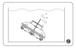
Hold the handle and put it vertically into the pool and fully submerge the device.
