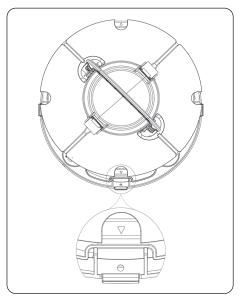
When fastening the top cover and chassis, please focus more on the installation direction as shown in the left figure: you shall ensure the arrow position marked on the cover buckle be aligned with the hole position, and insert pin on the top cover into hole.
