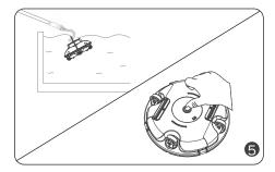
Insert the included hook into a pool pole and lift the cleaner out of the pool. Remember to power off the device.
