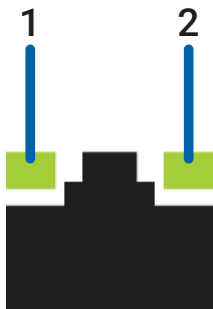
Figure 7: (1) Link LED. (2) Connection activity LED.
