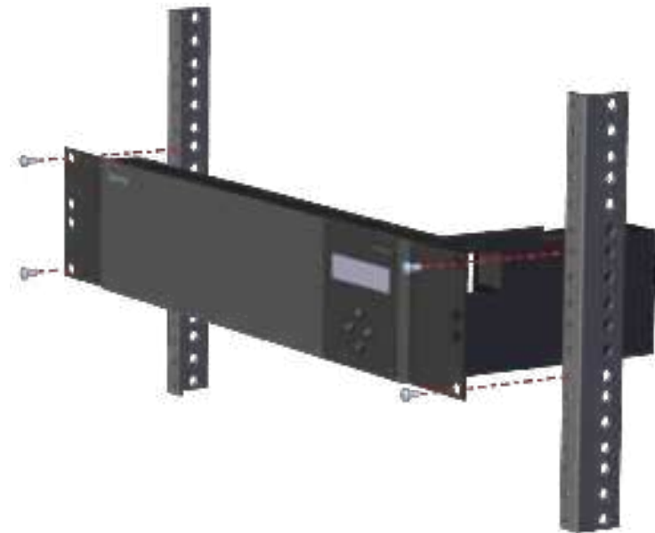
Figure 31. Attach controller assembly to the rack (hardware not provided)
