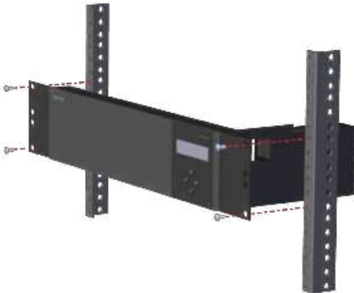
Figure 6. Attach the controller to the rack
