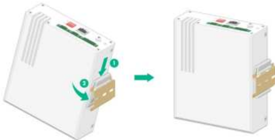
Figure2-3 Installing the switch on a DIN rail
