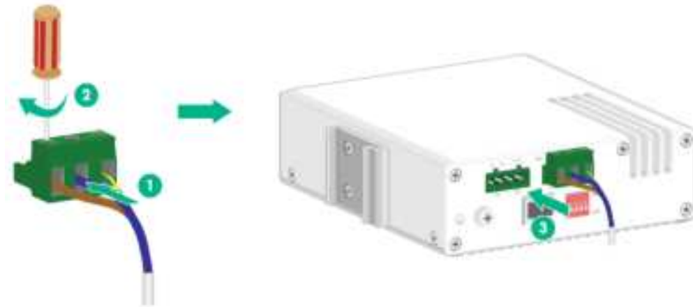
Figure2-7 Connecting an AC power cord for an SI 3100-8G-4S switch
