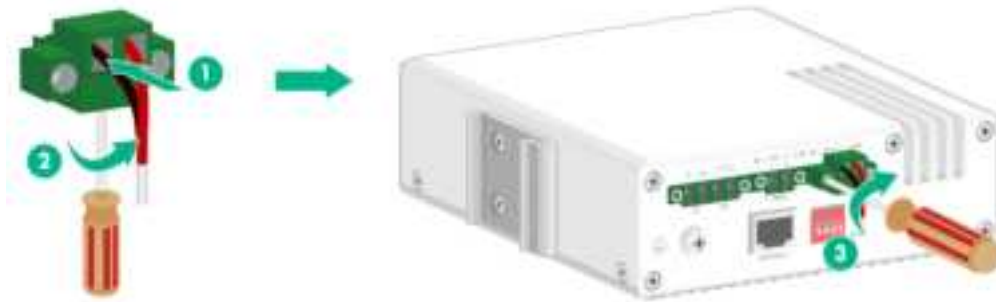
Figure2-8 Connecting a DC power cord for an SI 3100-8GP-4S switch
