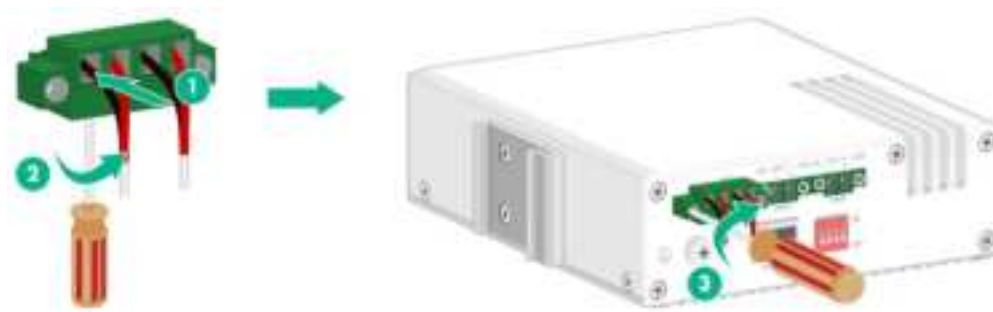
Figure2-6 Wiring external alarms for an SI 3100-8GP-4S switch
