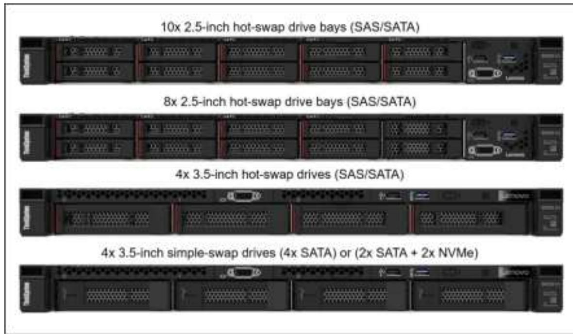
Figure 2. Front configurations of the ThinkSystem SR250 V3
