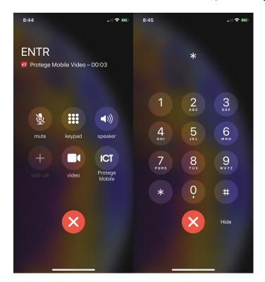
To view the video feed, press either the **video** or **Protege Mobile** button, then unlock the mobile device. This will launch the app and the **in app call screen** will be displayed.
