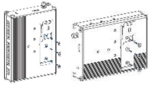
2. Hang the device to the DIN rail. The width of DIN rail is  $3.5 \mbox{cm}.$
