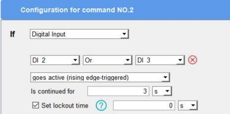
2. Set a IF condition based on the terminal device data or UC300 device status. Users can add at most 2 conditions in one command.
