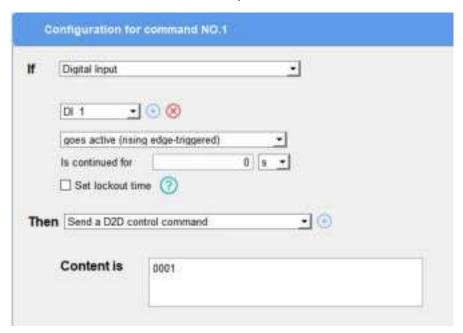
When UC300 receives a D2D command, it can work as a D2D agent to trigger the D0, restart the device or send Modbus command to RS485 terminal devices.
