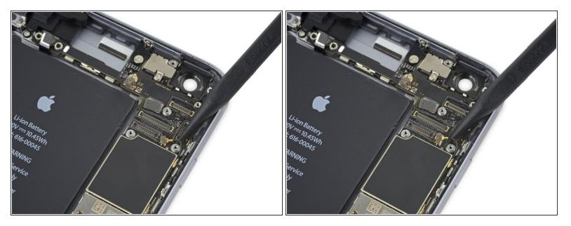
Disconnect the Wi-Fi diversity antenna cable by prying its connector up from the logic board.
