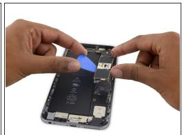
Carefully raise—but do **not** remove—the logic board, lifting it from the bottom edge nearest the Lightning connector.
