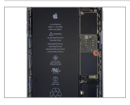
Remove the final 2.0 mm Phillips screw directly below the SIM card reader.
