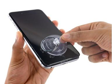
Pull up on the small nub on the suction cup to remove it from the display.
