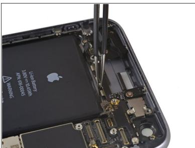
Deroute the upper left cellular antenna cable from the first logic board clip by nudging it out from under the clip, towards the battery.
