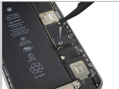
Remove the battery connector bracket.
