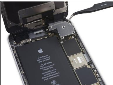
Remove the display cable bracket.
