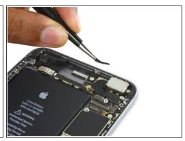
Peel up any tape covering the iSight camera bracket screws.
