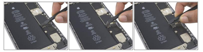
Bend the connector back to ensure it doesn't make contact and power the iPhone on while you're working on it.
