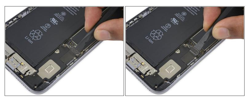
Use the flat end of a spudger to disconnect the Lightning connector flex cable from the logic board.
