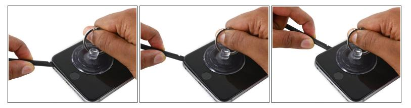
While firmly pulling up on the suction cup, slide the edge of the spudger under the bottom left corner of the display.
