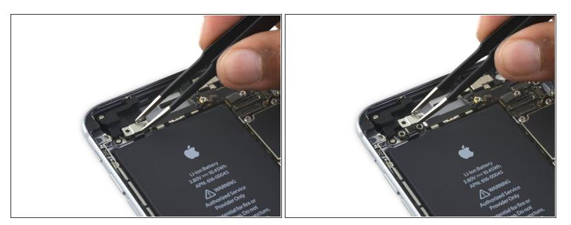
Remove the audio control cable bracket.
