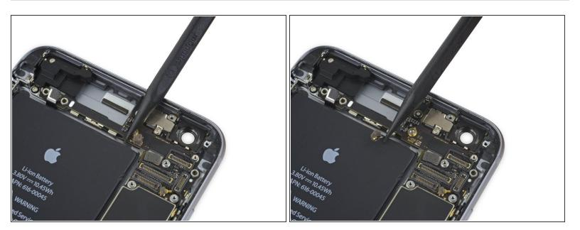
Disconnect the cellular antenna cable by prying its connector straight up from its respective socket on the logic board.
