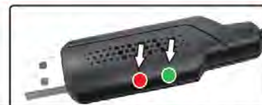
Battery pack having been fully charged, both Red and Green LED are solid on.
