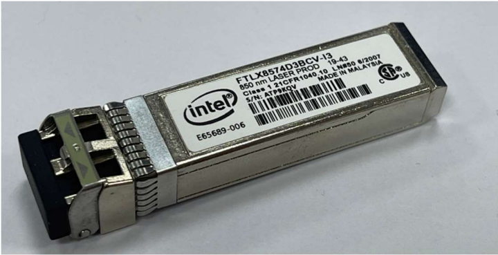
Figure 4 Accessories - 10Gb SFP+ optics, multi-mode
