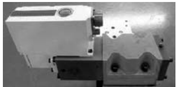
Figure 5. Mount the AxisPro valve to the adaptor plate.
