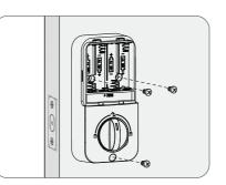
Secure the interior assembly with the supplied screws.
