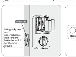
While the door is open and unlock, load 3AA batteries into the interior assembly.
