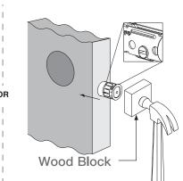
IMPORTANT: Keep the latch in unlocked position before installation.
