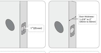
infirm that the hole in the door is Measure to confirm that door thickness is between 1–3/8" and 2" (35mm to 50mm).
