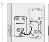
Remove the battery cover. | Connect the cable and ensure tight cable connection.
