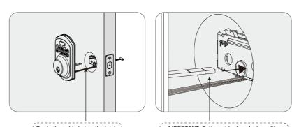
Route the cable below the latch. | IMPORTANT: Bolt must be in unlock position | Note horizontal orientation of tourque blade.
