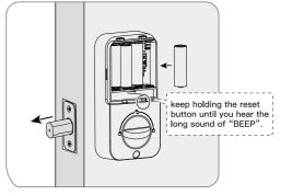
Keep holding the reset button, and load the last battery. Hold the reset button until you hear the long sound of "BEEP". The lock will automatically go into locking position. This is for the smart lock to memorize the orientation of the door.
