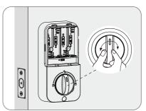
Test the lock by rotating the thumb turn to see if the bolt can be extended and retracted
