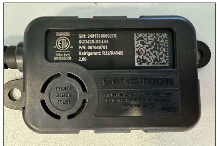
FIGURE 21. Example of Clear, Unobstructed Sensor Inlet
