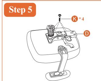
Attach Mechanism **(D)** to the Seat Cushion **(B)** with Bolts **(K)\*4**.
