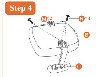
Turn the Seat **(B)** upside down. Install Armrests **(C)**\*1L\*1R to the Seat **(B)** with Bolts (M)\*2 and **(N)**\*4.
