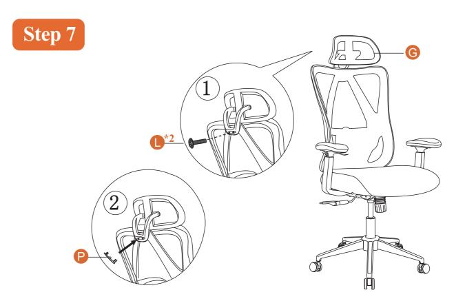
Using Wrench (Q), attach Head Pillow (G) to the Backrest (A) with Bolts (L)\*2. Then, attach the Plastic Cover (P) to the hole.
