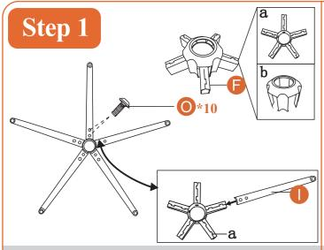
Divide Base (F) into two parts, a and b. Using Wrench (Q), install Legs (I)\*5 to the Base (a) with Bolts (O)\*10.
