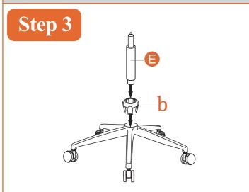
Put Base Cover **(b)** back on the Base. Then insert Gas Lift **(E)** into the center hole of the Base **(F)**.
