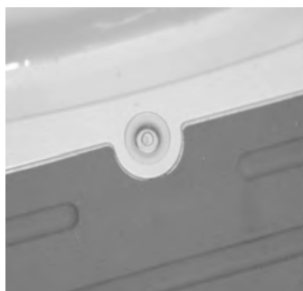
Figure 2-9. Bubble Indicates Scale Is Level
