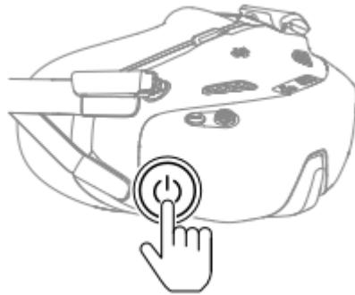
Press the power button once to check the current battery level.
