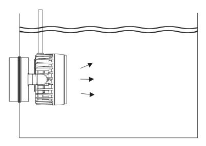
• Place the pump at least 3 inches(7-8CM) underwater and attach it to the outer glass of the aquarium using the magnetic holder.
