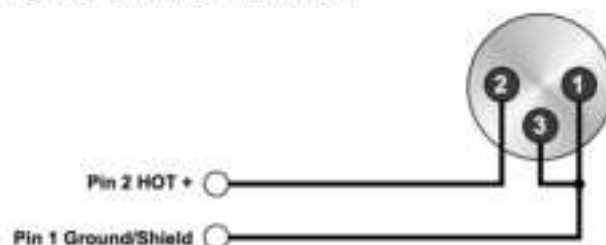
Input XLR Unbalanced Connection
