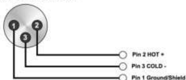
Output XLR Balanced Connection
