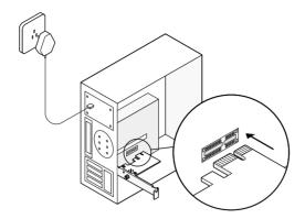
5. Locate an available F\_USB connector and carefully plug the Bluetooth USB cable into it.
