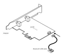
4. Locate an available PCIE slot (X1, X4, X8, or X16) and carefully insert the adapter.
