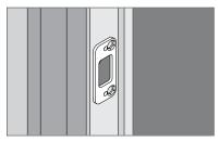
4b If correction is necessary, trace faceplate and mark holes.
