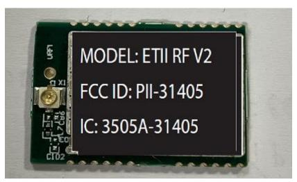
The label is placed on the shield. Any product that incorporates this module will have a label on the outside of the enclosure that includes the following wording:
