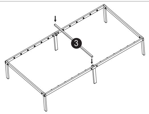
Insert Center Slat (3)\*1 onto the **groove** in the middle of the Side Frame (2)\*2.
