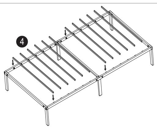
Insert Slats (4)\*12 evenly onto each groove of the Side Frame (2)\*2.
