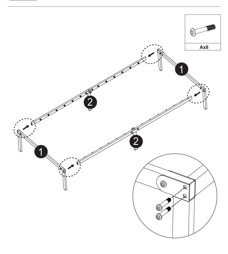
Attach Side Frame (2)\*2 to the four corners of the Frame (1)\*2 with Screws (A)\*8.
