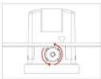
Rotating output gear will drive the gate frame.
