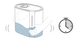
3 Place the tank on the base, vinegar mixture will drain into the reservoir. Soak for another 15 to 20 minutes.
