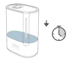
4 Remove the tank from the base, and pour out any vinegar mixture from the reservoir and tank.
