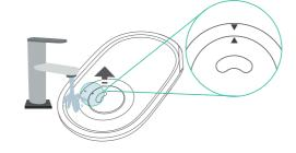
2 Remove the water tank from the base. Pour out any water from the reservoir. Do not allow liquid to enter the air outlet.
