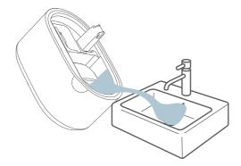
3 Remove the water filter from the tank by rotating it counterclockwise and lifting it out.
