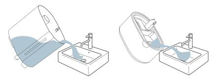
5 Use a soft cloth and the cleaning brush to remove scale from all parts. Rinse with room temperature water.
