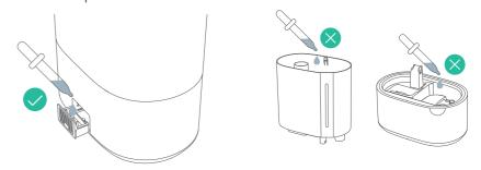
5 Plug in the humidifier. Tap Power Button to turn on. The humidifier will start misting.
