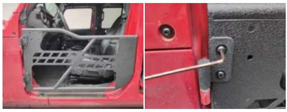
Loose the lock cover. Adjust the lock.
