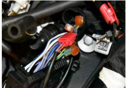
Splice the SH Black wire to the Black wire of the fan connector. Use a red wire tap connector.
