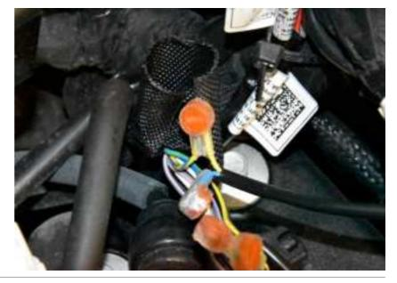
Splice the SH Red wire to the Grey/Pink wire of the ABS connector. Use a red wire tap connector.
