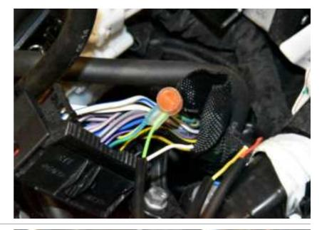
Connect the SH Blue wire to the Green/Blue wire end, which is at the wiring harness side. Use a yellow butt connector.
