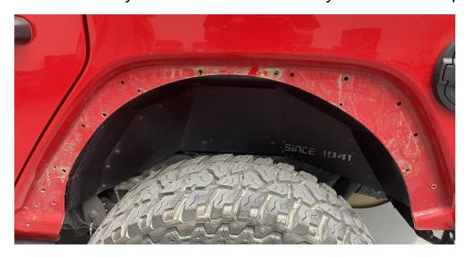
Step 6: Install the rivet nut into the four holes with the rivet nut tool.
