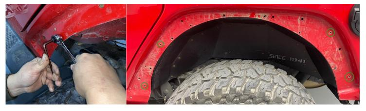
Step 7: Install the rear fender flare. Use the Button Head Socket Cap Bolts Screws (M6\*35), Split Lock Washer (D6), Flat Washer (M6\*16\*1). Only the upper installation holes need use the Flange Hex Lock Nuts(M6). Tighten up those bolts.
