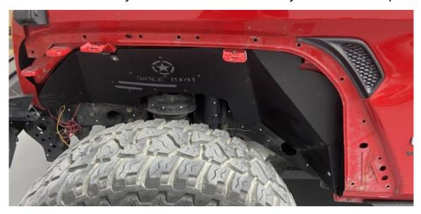
Step 2: Install the rivet nut in the most right hole with the rivet nut tool.
