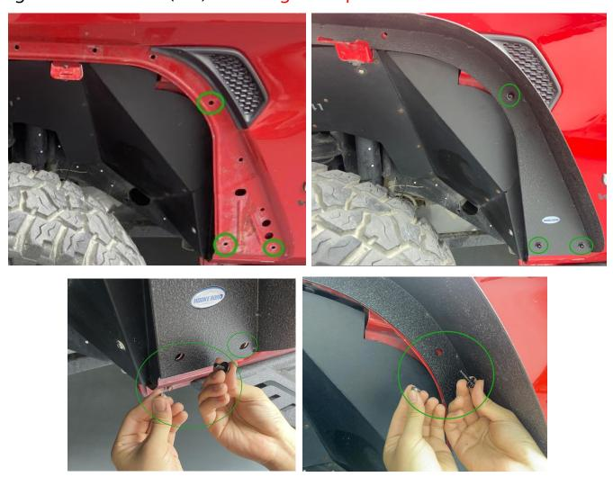
Step 4: Next, Install the connecting brackets (A&B&C) in order (Attention to distinguish the driver side and passenger side). Use the Button Head Socket Cap Bolts Screws (M6\*20), Flat Washer (M6\*16\*1), Flange Hex Lock Nuts (M6). Tighten up this step and the step 3 bolts.
