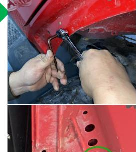
Step 3: Next, Lift up the front fender flare and install the right three holes. Use the Button Head Socket Cap Bolts Screws (M8\*20), Flat Washer (M8\*16\*1), Flange Hex Lock Nuts (M8). Don't tighten up those bolts.
