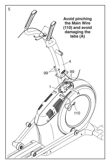
Locate the wire tie (B) in the lower end of the Upright (4). Tie the wire tie to the Main Wire (110). Then, pull the upper end of the wire tie until the Main Wire is routed through the Upright.
