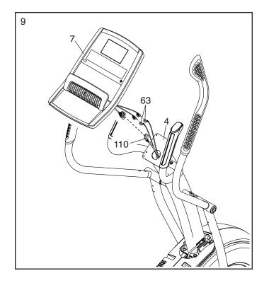
10. **Tip: Avoid pinching the wires.** Attach the Console (7) to the Upright (4) with four M4 x 16mm Screws (101); **start all the Screws, and then tighten them.**
