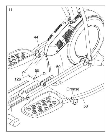
12. Apply grease a Pedal Arm Axle (64).
