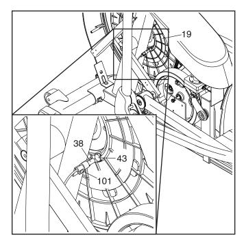
Next, slightly loosen the indicated M4 x 16mm Screw (101), slide the Reed Switch (38) slightly closer to or away from the Magnet (43), and then retighten the Screw. Then, plug in the power cord, press the power switch to the reset position, and rock the Pulley (19) forward and backward just enough that the Magnet passes the Reed Switch repeatedly.
