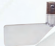
PDL-4. 316 SS single vane paddle for heavy weight materials with a minimum bulk density of 70 lb/ft³ (1122 kg/m³). Fits through 1-1/4" coupling eliminating the need for a mounting flange.
