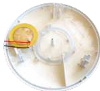
Excessive dust inside alarm
