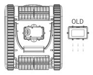
b. Insert the new battery according to the corresponding contacting positions of used battery.
