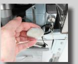
• Open left door and pull dispose valve handle.
