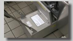
• Place water removal caddy capable of holding four gallons under fryer at prompt and tap Yes.
