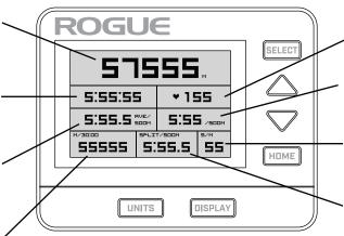
Display your heartrate if M2 is connected to a heartrate belt and you are wearing this heartrate belt correctly.
