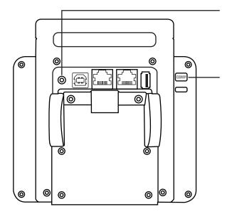
Combination buttons to realize reset function press button unit and display at the same time, then poke reset, hold them for 7 second, screen display "setting factory defaults", release buttons will enter reset.
