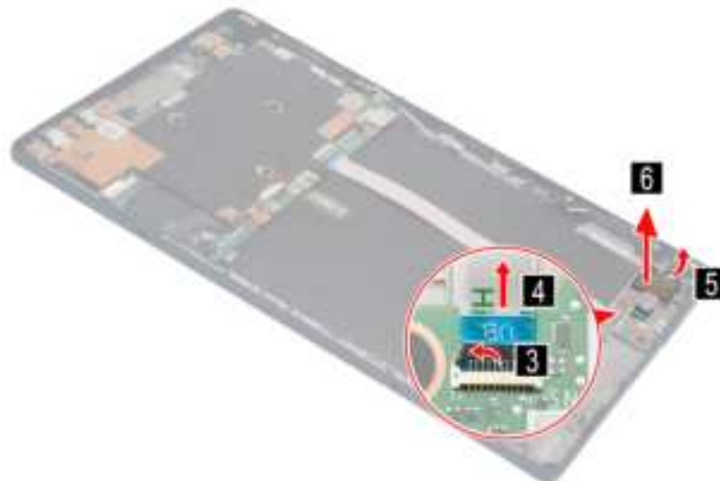
Figure 10. Disconnect the fingerprint board cable and then remove the fingerprint board
