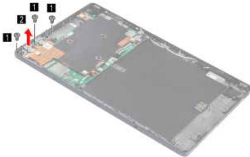
Figure 22. Remove three screws and the Type-C bracket
