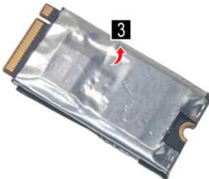
Figure 19. Remove the solid-state drive foil
