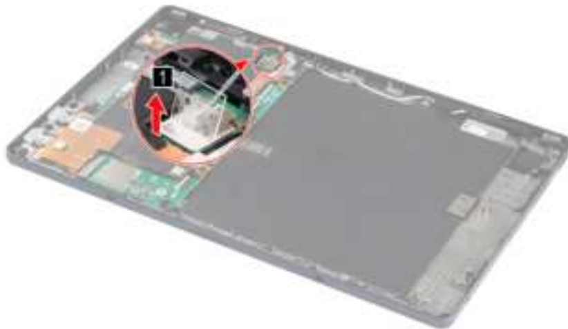
Figure 20. Remove the the WLAN mylar
