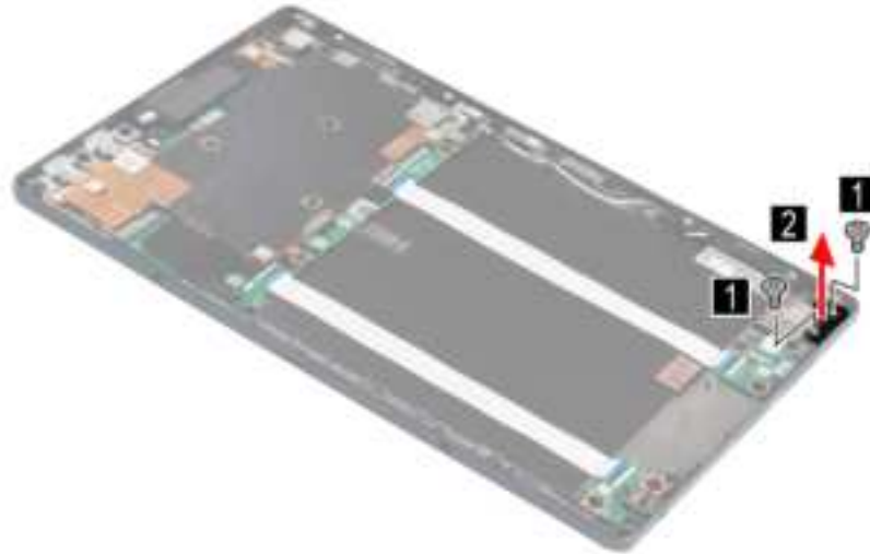
Figure 9. Remove two screws and the fingerprint board holder
