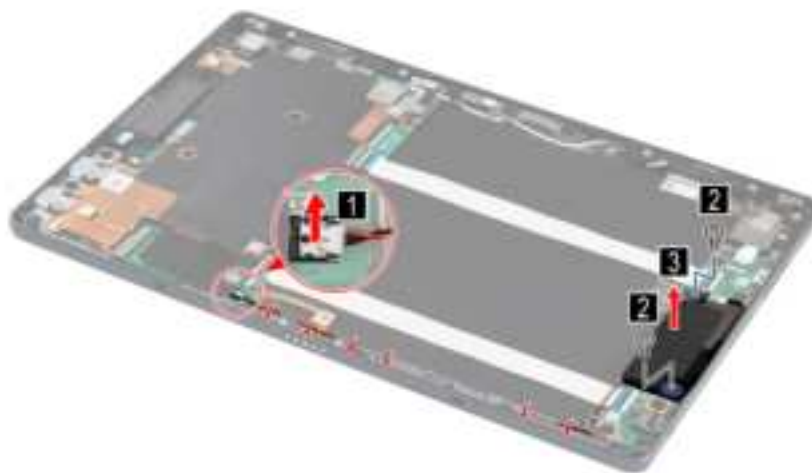
Figure 6. Disconnect the speaker cables, remove two screws and the speaker
