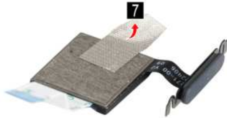
Figure 11. Remove the fingerprint conductive tape from the fingerprint board
