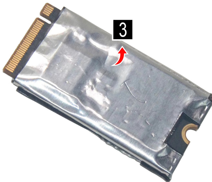
Figure 19. Remove the solid-state drive foil
