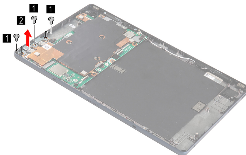
Figure 22. Remove three screws and the Type-C bracket
