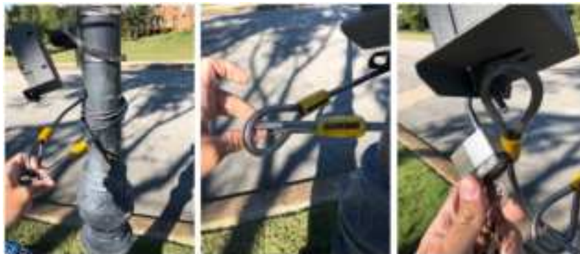
Figure 17: Locking the Cable Lock
