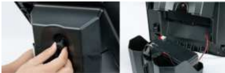
Figure 8: Exposing the Battery Compartment
