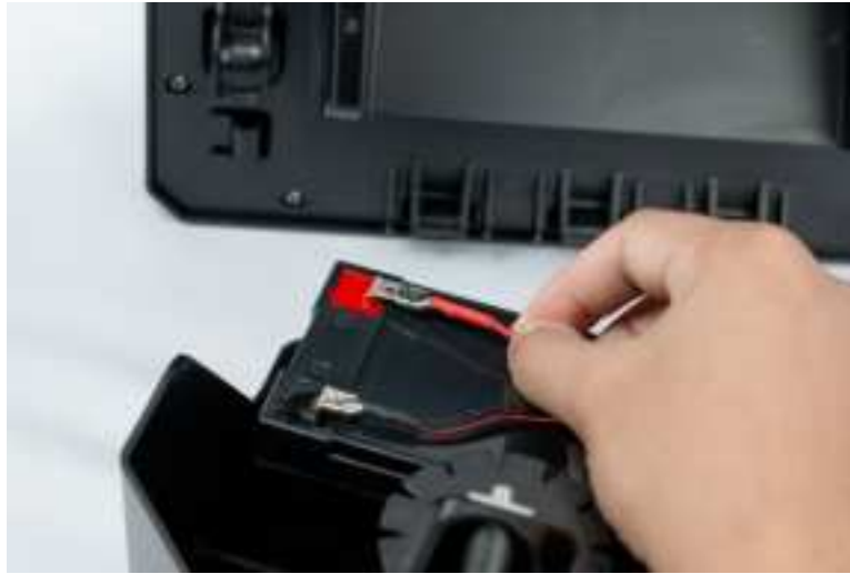
Figure 9: Connecting the Battery Terminal
