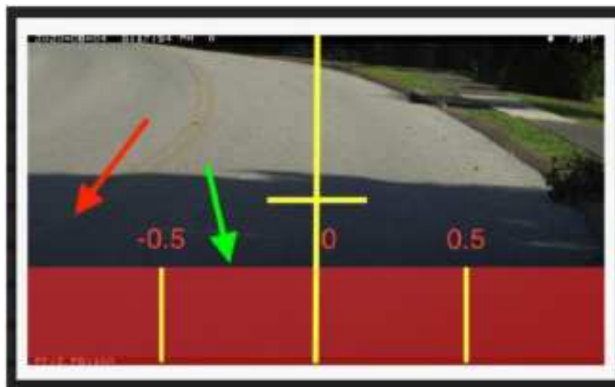
Figure 21: Adjusting Camera Aiming Point
