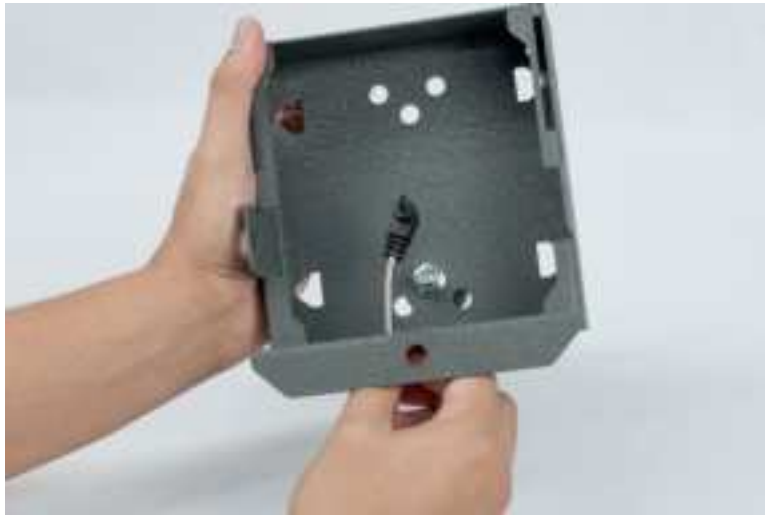
Figure 7: Power Cable Female Connector End
