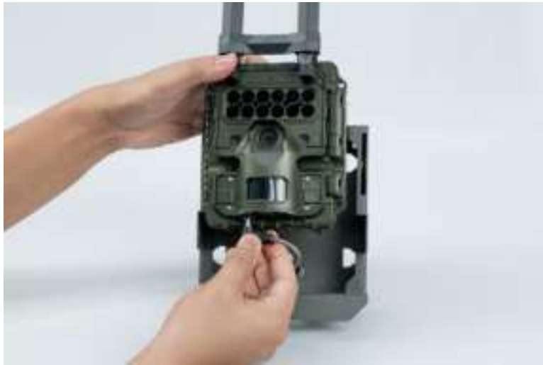
Figure 15: Plug in the Power Cable
