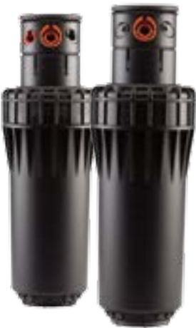
I-90 Overall height: ADV/36V: 28 cm Pop-up height: 8 cm Exposed diameter: 9 cm Inlet size: 1½" (40 mm) BSP
