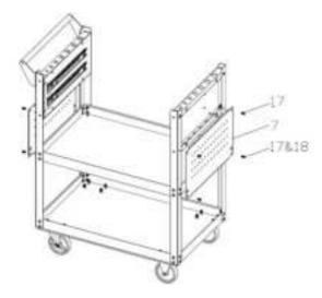
Step 6: Assembly the Beam 9# and Back board 11# with Bolt 17#.
