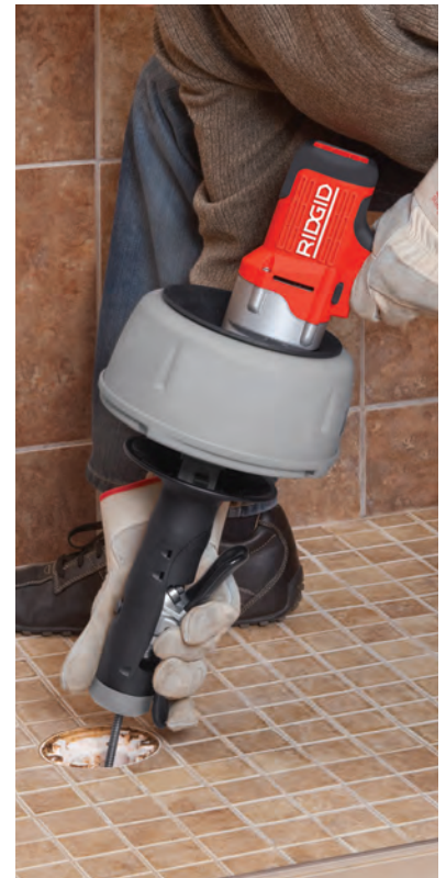
The ¾" cable in Model K-45AF-5 and K-45AF-7 extends machine's capacity to 2½" drain lines.
