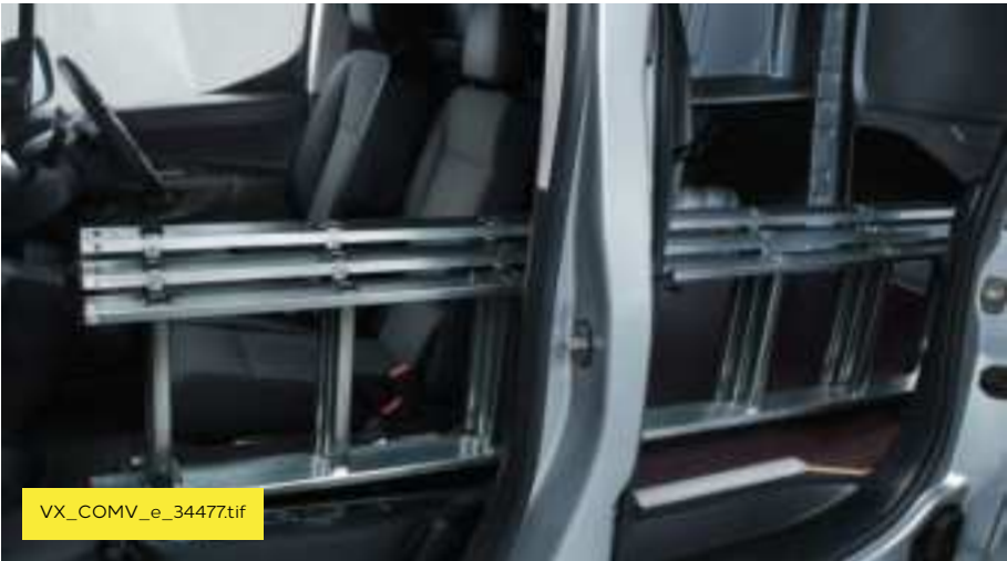
Load-through hatch within bulkhead
