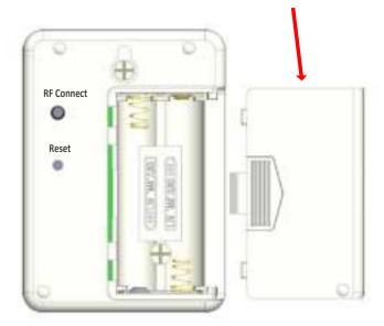
Press and hold "RF Connect" for 5 seconds enter pairing mode.
