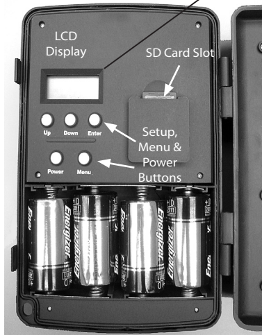
Control Panel (Front Opened)
