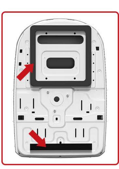
Take out one gasket and one sponge with sealing strip. Stick the gasket and sponge to the fixed positions on the outdoor unit chassis.
