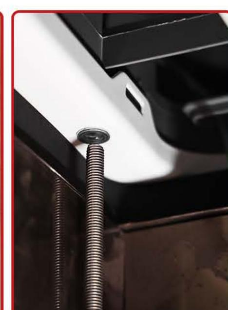
If the roof thickness is between 1.2-3.15 inches, use the provided 5.3" mounting bolts to secure the ceiling frame to the rooftop air conditioner. For roof thickness between 3.15-5.32 inches, please use 7.5" bolts (not included).
