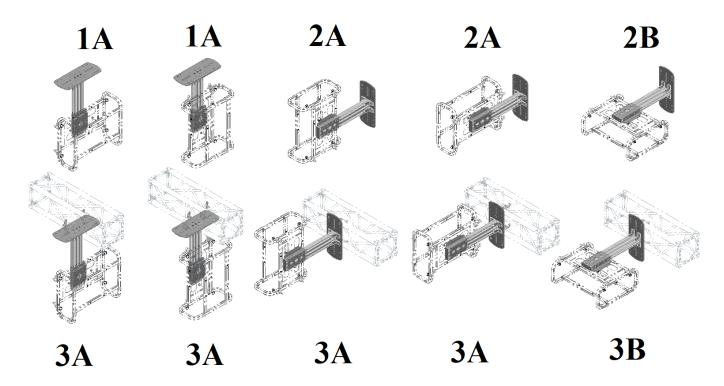
N.B: In all installations where the profile is mounted parallel to the floor (wall installation or in some cases truss), make sure the plate is mounted with the longer side perpendicular to the floor, as this will ensure more stability.
