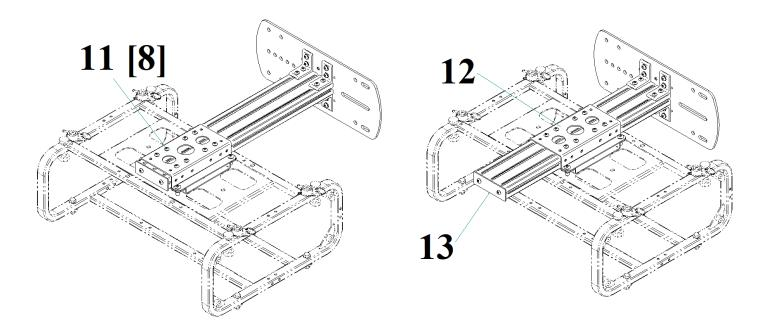
N.B: ARM is equipped with a safety limit switch (13) so that the product is safe under all conditions (even if the profile is vertical and therefore the support could fall due to gravity after the screws (11) have been loosened could fall).
