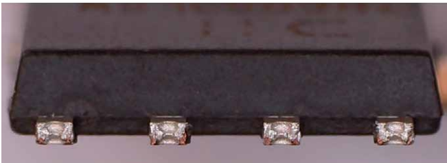
Lead sidewall dimple feature on the PowerDI5060-8 package
