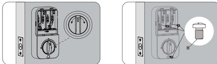
**IMPORTANT:** Lock knob will only rotate to the lock position in either the clockwise or counterclockwise direction based on your door handing, not both.
