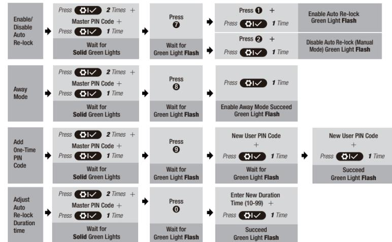
**NOTE:** When setting unsuccessful, the indicator light will flash red. If no button is pressed for more than 10 seconds, the lock will exit programming mode.
