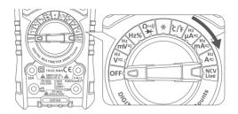
Note: Use the "FUNC" Button to select a specific function if there are multiple functions in one rotary setting.
